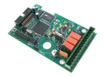
The Xtralis VESDA VLF MCC (Multi-function Control Card) is an interface card for the range of Xtralis VESDA VLF smoke detectors. An MCC expands the range of input and output communications a VLF can perform.
