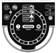
When the field service access door is open, the user has access to the RESET (5, DISABLE 1, Fire Test 1 AutoLearn 1) and Instant Fault Finder functions. When the Instant Fault Finder function is activated, the Smoke Dial converts to a fault indicator, with the dial segment numbers corresponding to the faults listed below.
