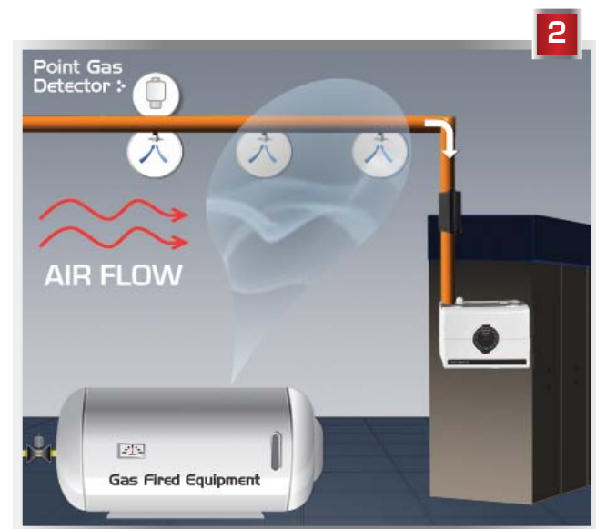
Figures 3 + 4 – Demonstrate the design flexibility of VESDA ECO. Knowing where a leak will occur is always a judgement call. In this example, four conventional point gas detectors are required to cover the same area as one VESDA ECO detector. VESDA ECO provides a more cost-effective solution.
