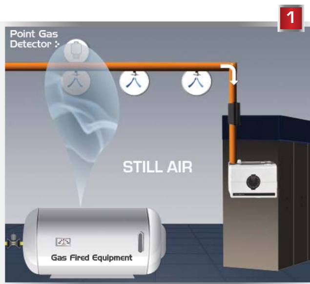
Figures 3 + 4 – Demonstrate the design flexibility of VESDA ECO. Knowing where a leak will occur is always a judgement call. In this example, four conventional point gas detectors are required to cover the same area as one VESDA ECO detector. VESDA ECO provides a more cost-effective solution.
