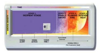
A Xtralis VESDA smoke detector can be configured to detect a fire at the earliest stage. The multiple alarm levels can be configured to initiate an appropriate response at all stages of a fire.
