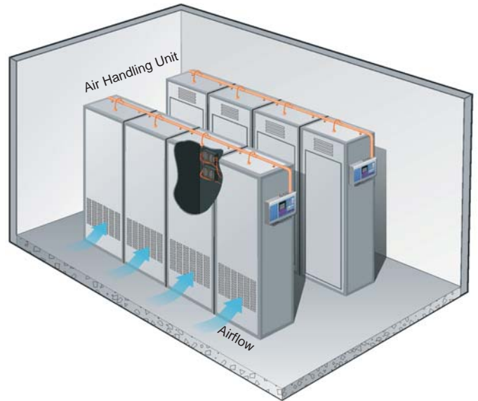
Fig 4. In-Cabinet Capillary Sampling for Switch Rooms
